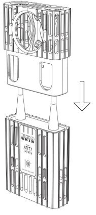
2. slide over the antennas and insert the top cover and push it in to the bottom.
