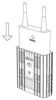
**1.** insert the AsteraBox and push it to the bottom.
