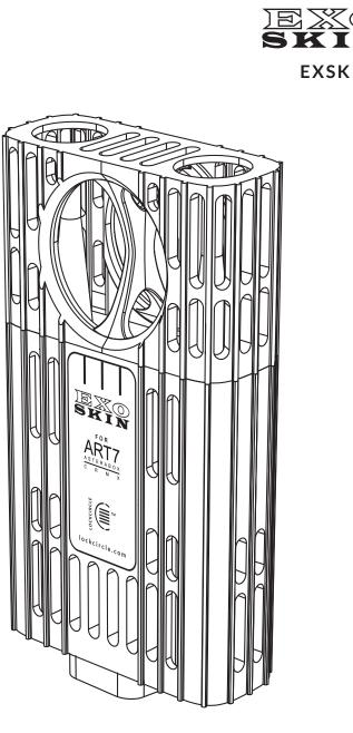
The Exo Skin is a protective casing to protect the Astera Box during tough daywork production day. Manufactured with carbon fiber additive technology for strong impact and drop resistance. A CNC Machined Aluminium L-Bracket with vertical and horizontal threads (2x 1/4-20 / 2x 3/8-16) allows it to be clamped securely.
