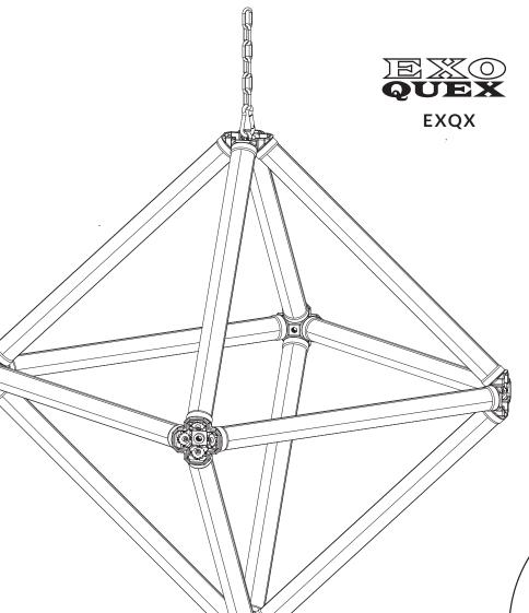
The Exo Quex was designed to create diamond shapes with Astera Titan and Helios LED tubes, but with the Exo Quet can be created square pyramids. Also the top mount is a 3/8"-16 thread, and for multiple layers "diamond in diamonds" or "pyramid in pyramids", can be used the bottom Mount.
