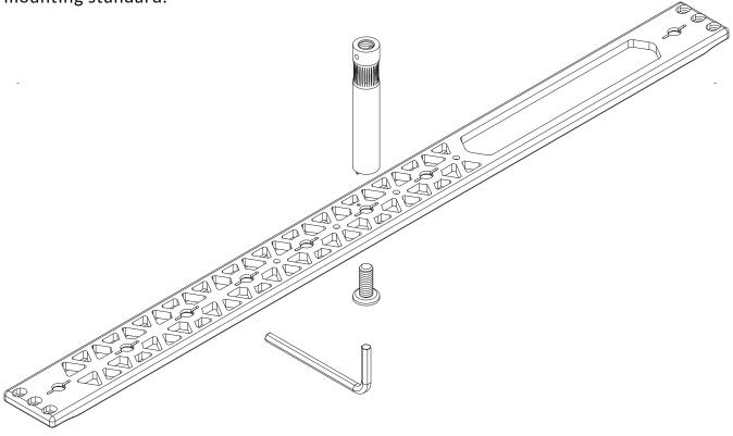
The pin has a 3/8" - 16 thread on top and is made of Grade 5 Titanium, with an exclusive SCK Straight Concave Knurling channel that allows extremely precise use. It is mounted with a bolt with a 3-Way fixing head (coin, screwdriver and Hex Tool), also in Titanium.
