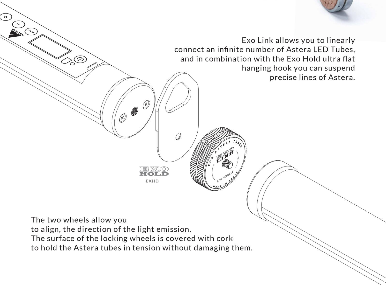
The two wheels allow you to align, the direction of the light emission.
