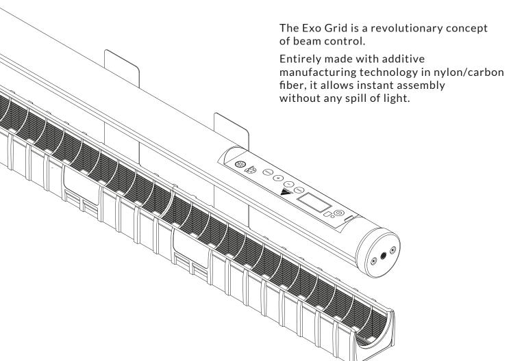
The inner part of the grid is made with a "dielectric pattern" to offer an exclusive softness and nuance of light. Available in two versions at 60° and 45°, and in the kit with neoprene pouch, supplied with two nano-Velcro straps for extra safety (however the grid hooks with force) for use on moving cars, motorboats or other. The Exo Grid works on any Astera Helios or Titan tube.
